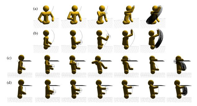
Fig. 5. Results of probabilistic inference planning with an humanoid upper body. (a&b) Reaching to a target without obstacles, displayed from two different perspectives. We see the MAP joint configuration and the Gaussian endeffector distribution (indicated as ellipsoid) at different intermediate time steps. The optimal trajectory in joint space leads to a curve trajectory in endeffector space. (c) Reaching to a target above the table and (d) below the table whilst avoiding collision.
