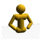
Fig. 1. A humanoid upper body with n=13 hinge joints. The hip is fixed, the right hand is used as endeffector.
