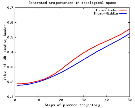
Fig. 7. A complex grasping trajectory in configuration space is represented by a pair of simple monotonically increasing curves in our topologically motivated state space consisting of  $y_t = (\hat{w}(\gamma_1(t)), \hat{w}(\gamma_2(t)))$ . The graph displays steps  $t$  in the simulation (horizontal axis) against the values of  $\hat{w}(\gamma_1(t))$  and  $\hat{w}(\gamma_2(t))$ .
