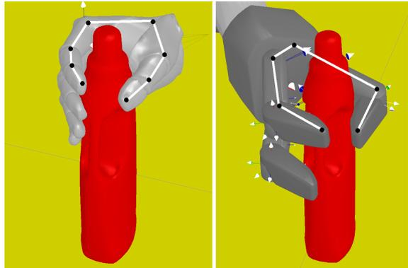
Fig. 1. Demonstrated stable human grasp (left) and transferred grasp (right) applying our topological approach
