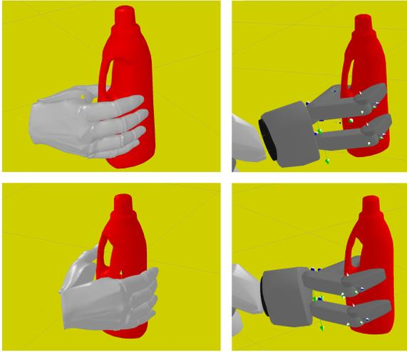
Fig. 5. Left side: examples of bottle grasps generated with human-like hand. Right side: Results of motion planning with a 3-finger Schunk hand.
