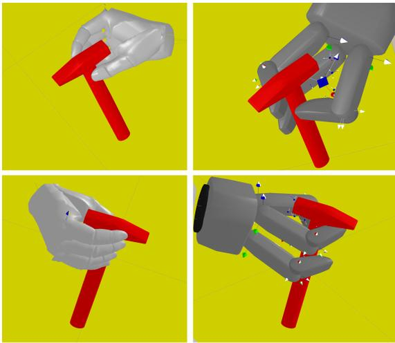
Fig. 6. Left side: examples of hammer grasps generated with human-like hand. Right side: Results of motion planning with a 3-finger Schunk hand.
