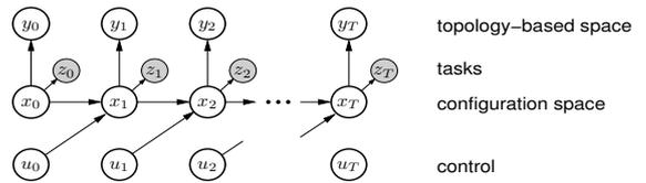
Fig. 4. AICO in configuration and topology-based space. The new topology motivated space represented as an additional task variable.
