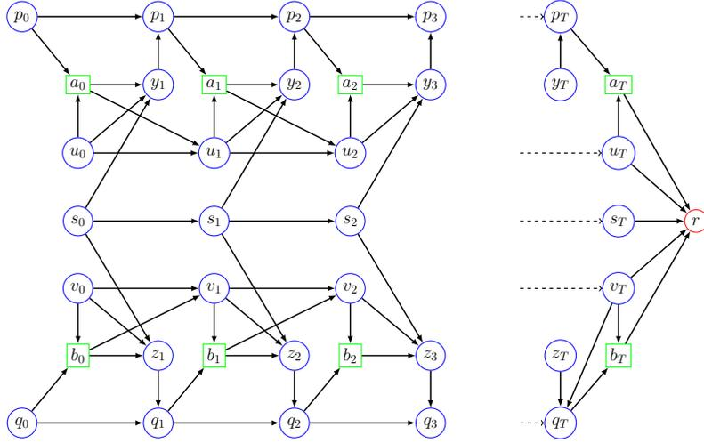
Figure 13: A T-step DBN for a link involving two agents. There is one such DBN for each link  $l$  and every time step  $T$ . In top three layers,  $p$  denotes first agent's (on link  $l$ ) controller nodes,  $a$  denotes action and  $u$  denotes internal state. The layer  $s_i$  denotes the external state. In bottom three layers,  $q$  denotes second agent's controller nodes,  $b$  denotes action and  $v$  denotes the internal state
