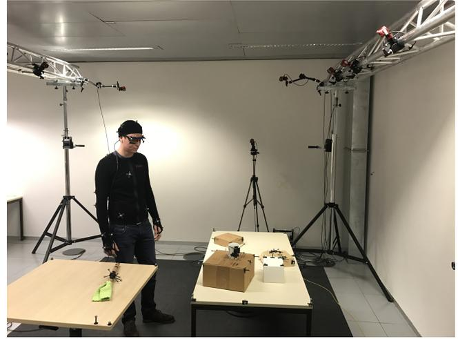
Fig. 3: Motion capture system used in the experiments.
