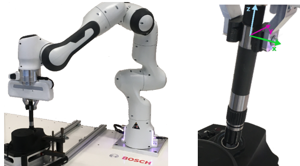
Fig. 1. Left: the Franka Emika Panda robot employed for fitting an eBike motor shaft into a ball-bearing located in the motor housing. Right: a close-up view on the shaft.
